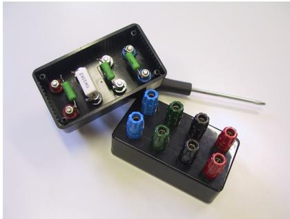
**Figure 1:** Resistor box.
