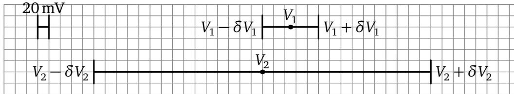
**Figure 8:** To check the compatibility between two measurements  $V_1$  and  $V_2$ , with uncertainties  $\delta V_1$  and  $\delta V_2$ , respectively, draw to scale the two values with the corresponding uncertainty bars, which should overlap.
