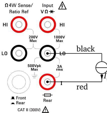
**Figure 10:** To measure a DC current with the Agilent 34401A multimeter, connect the red test lead to the *Input I* terminal and the black test lead to the *Input LO* terminal. Then, connect the test leads *in series* with a branch of the circuit under test, here represented by the current source  $I_s$ . (§2.1)
