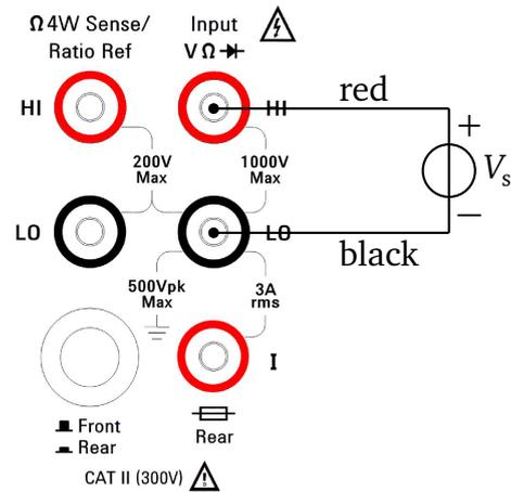
**Figure 6:** To measure a DC voltage with the Agilent 34401A multimeter, connect the red test lead to the *Input HI* terminal and the black test lead to the *Input LO* terminal (colours are assigned conventionally). Then, connect the test leads *across* two points of the circuit under test (e.g. the two output terminals of the power supply), here represented by the voltage source  $V_s$ . The *Input LO* terminal is the reference terminal for voltage and current measurements. (§1.1)
