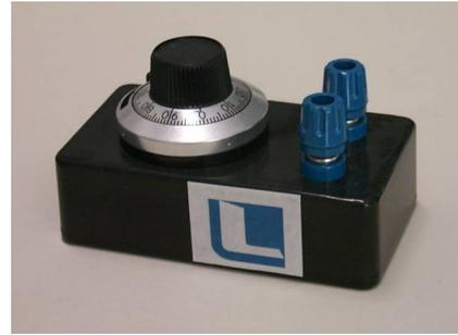
**Figure 2:** Variable resistor.
