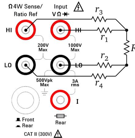
**Figure 15:** In a four-wire resistance measurement, the multimeter uses the *Input* terminals to inject a current through  $r_1$ ,  $R$  and  $r_2$ , and uses the *Sense* terminals to measure the voltage directly across  $R$ . The voltage drop across resistances  $r_3$  and  $r_4$  is negligible because the current flowing into the *Sense* terminals is virtually zero. (§3.1.2)
