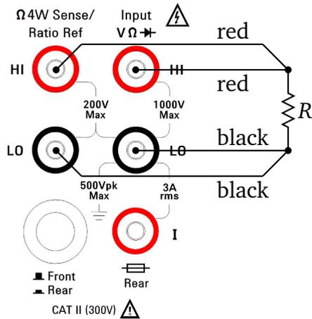
**Figure 14:** Four-wire resistance measurements with the Agilent 34401A: the *Input HI* and the *Sense HI* terminals should be connected to one of the resistor terminals; the *Input LO* and the *Sense LO* terminals should be connected to the other resistor terminal. (§3.1.2)
