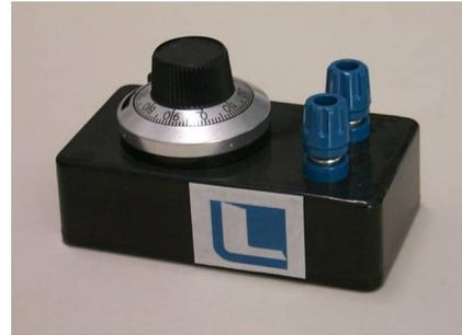
**Figure 2:** Variable resistor.
