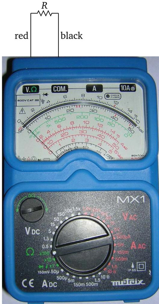
**Figure 16:** To measure a resistance with the Metrix MX1 multimeter, connect the red test lead to the  $V.\Omega$  terminal and the black test lead to the  $COM.$  terminal. (§3.2)
