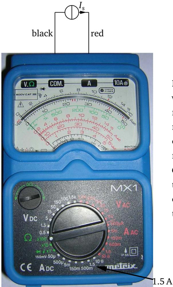
**Figure 11:** To measure a DC current with the Metrix MX1 multimeter, you must firstly select the proper range manually (1.5 A in this case). Next, connect the red test lead to the A terminal and the black test lead to the COM. terminal. Finally, connect the test leads *in series* with a branch of the circuit under test, here represented by the current source  $I_s$ . (§2.2)
