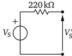
**Figure 9:** Circuit to test the effect of voltmeter loading.
