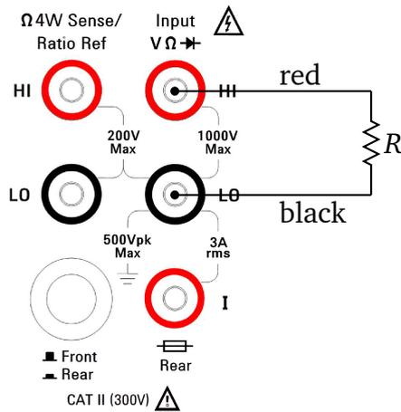
**Figure 12:** Two-wire resistance measurements with the Agilent 34401A: connect the red test lead to the *Input HI* terminal and the black test lead to the *Input LO* terminal. Then, connect the two leads to the unknown resistance  $R$ . (§3.1.1)
