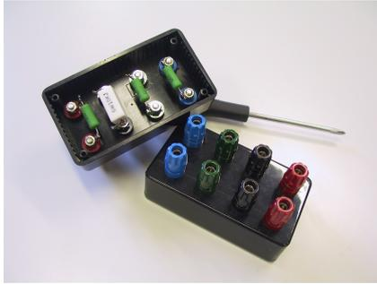
**Figure 1:** Resistor box.
