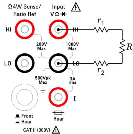
**Figure 13:** In a two-wire resistance measurement, the multimeter actually measures the sum  $R + r_1 + r_2$ , where  $r_1$  and  $r_2$  are the lead wire and contact resistances. (§3.1.1)
