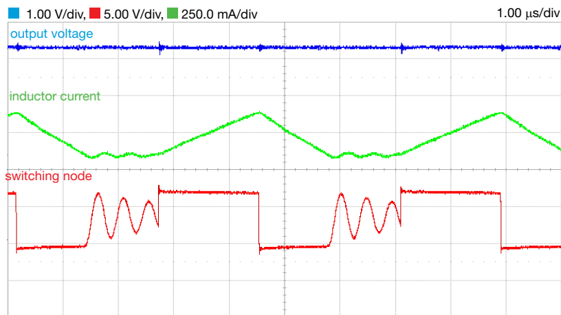
Figure 7. V_{in}=6V , I_{out}=0.1A , f_s=250kHz
